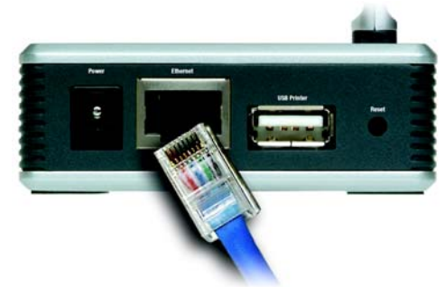
Figure 3-1: Connect to the Ethernet Port
