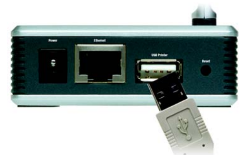
Figure 3-2: Connect to the USB Port
