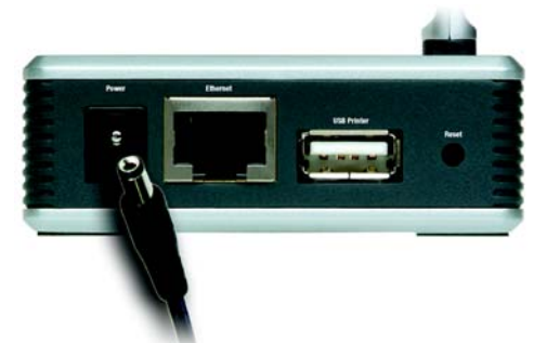
Figure 3-3: Connect to the Power Port
