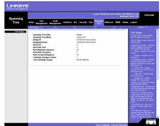
Figure 5-46: Spanning Tree - STP Status
