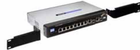
Figure 3-2: Attach the Brackets to the Switch
