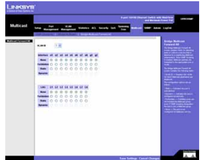
Figure 5-55: Multicast - Bridge Multicast Forward All
