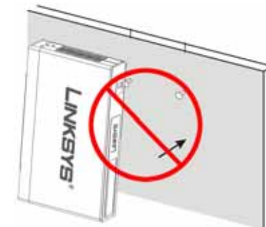
Figure 3-5: Incorrect Wall-Mount Orientation (Vertical)
