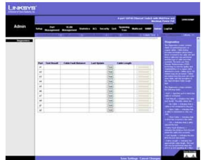
Figure 5-68: Admin - Cable Test
