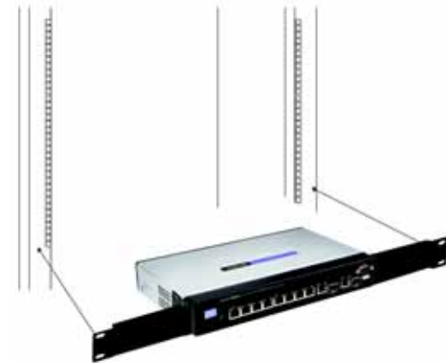
Figure 3-3: Mount the Switch in the Rack
