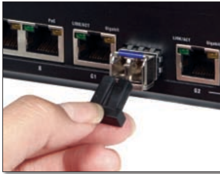
Remove the Rubber Port Cap
