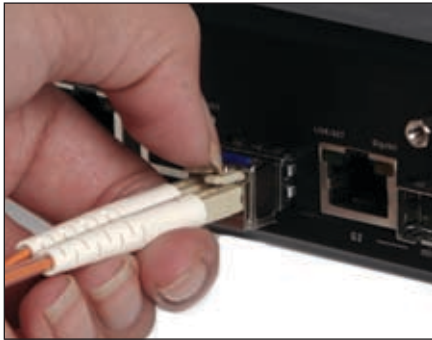
Remove the Fiber Cable
