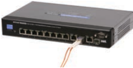
Connected Fiber Cable
